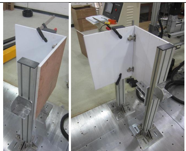
Pic. 8: Simulation test assembly for vertical hinge
