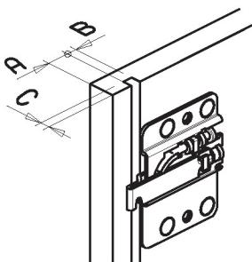
Position (A) and thickness of the back panel (B), depth of the milling (C).
