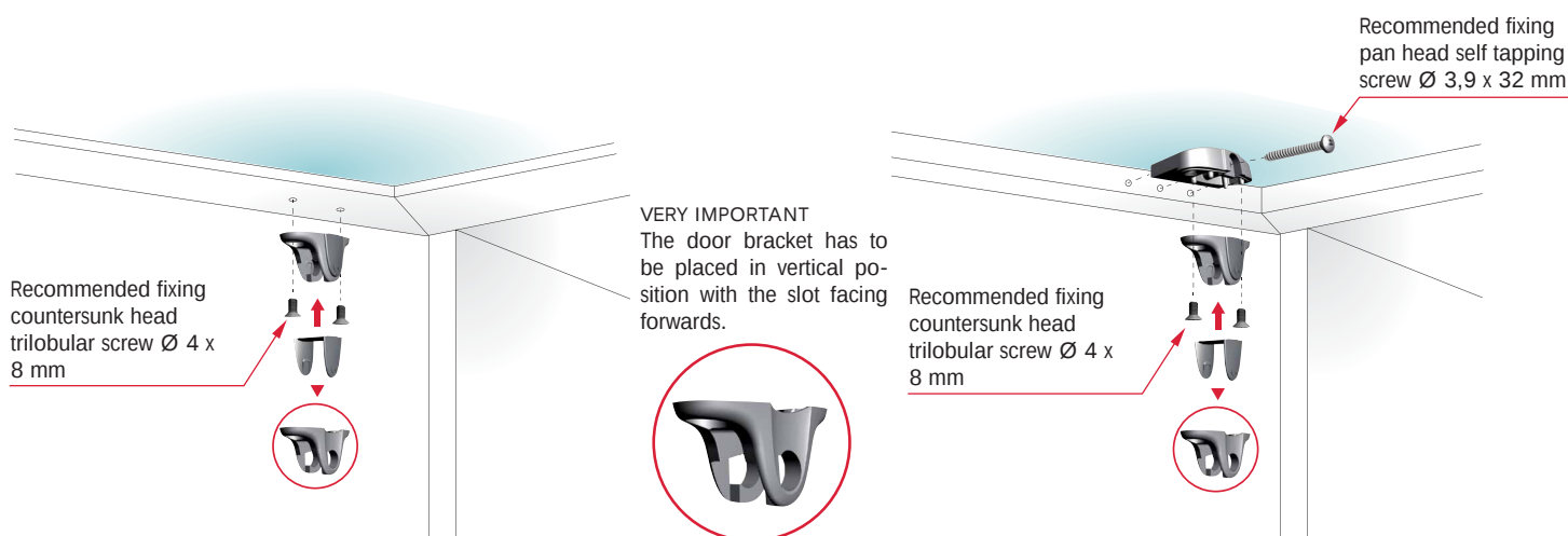
INSTALLATION ON WIDER ALUMINIUM FRAME DOOR
